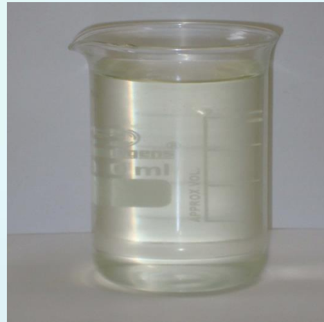
After Ozone Treatment & Post Filtration
